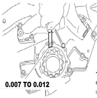
INSTALL THE OIL PUMP HOUSING AND ROTOR SET ON THE ENGINE. USING A FEELER GAUGE, MEASURE THE CLEARANCE BETWEEN THE OUTER ROTOR AND THE OIL PUMP HOUSING. MEASURE AT 4 LOCATIONS, 90° FROM EACH OTHER. THE MEASUREMENT MUST BE BETWEEN 0.007 AND 0.012.
