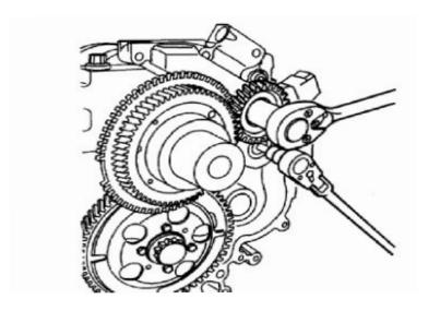
While holding the oil pump idler gear shaft with a hex driver, as shown in above figure, tighten the oil pump drive gear nut to 74 FT LBS.
